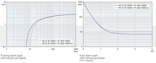
Pumping speeds and pump down times are only for information. Ultimate vacuum specification: See "Technical Data"
